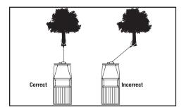
Short pulls from an angle can be used to straighten the vehicle. Long pulls should be done with the synthetic rope at a 90° angle to the winch/vehicle. When pulling a heavy load, place a blanket or jacket over the synthetic rope five or six feet from the hook.
