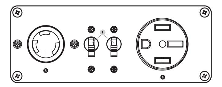
Circuit Breakers (flip Reset) – Protects the generator against electrical overloads.
