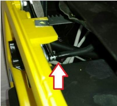
4. With the hoses disconnected, you can remove the 7mm fuel tank bolts and set the fuel tank aside.
