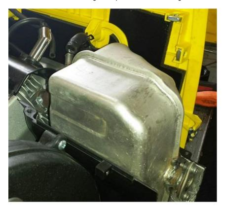
8. Remove the two 10mm bolts holding the muffler to the cylinder head.
