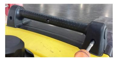
2. Remove maintenance panel and locate fuel drain hose. Place fuel drain hose into a safe fuel storage container and loosen drain screw. Turn fuel valve on to drain all gas from fuel tank.
