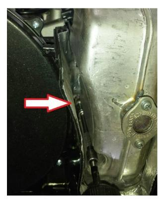
10. You can now remove the muffler and gasket.
