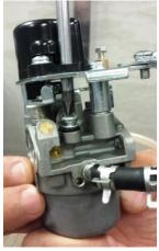
2. Using a small pocket screwdriver, lift the pilot jet an 1/8<sup>th</sup> of an inch in order to grab the jet with a pair of needle nose pliers. Use these to remove the jet from the carburetor.
