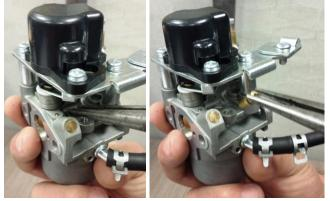
3. Using a strand of copper wire small enough to fit through the hole, clean the jet passage way. Then spray through the jet with carburetor or brake cleaner and then compressed air if available.
