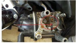
5. Reinstall pilot jet capture plate and Phillips head screw.
