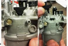
3. Using a strand of copper wire small enough to fit through the hole, clean the jet passage way. Then spray through the jet with carburetor or brake cleaner and then compressed air if available.
