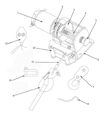
Motor: 1.34 HP 12V DC motor provides power to the planetary gear mechanism.
