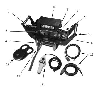
**Motor (1)**: 3.6 HP 12V DC motor provides power to the planetary gear mechanism. **Winch Drum (2)**: The winch drum is the cylinder on which the wire rope is stored. It can feed or wind the rope depending on the remote winch switch.
