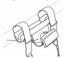
Double the strap over the ring and wrap back around the frame of the bicycle tightly. Wrap all the way around until the end of strap links with the tab. See image below.
