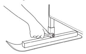
2. Attach both Support Rods (#5) to the Main Frame (#3) use one M8x65 Bolt (#12), one Flat Washer (#10) and one Locking Nut (#11)
