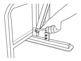
3. Put the Triangle Plates (#6) on each side of the Inner Post (#2). Slide one M8x50 Bolt (#12) through the Triangle Plates and Inner Post and secure with one Flat Washer (#10) and one Locking Nut (#11). Lightly oil the Inner Post (#2) and slide it through the post opening in the Main Frame (#3), NOTE: Make sure the Inner Post (#2) bolt sleeve is facing forward.
