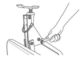
6. Once the Snowmobile Track Lift is put together make sure it is easy to use and slides up and down with minimal effort. If the lift is sticking or it is difficult for the Inner Post (#2) to move up and down, loosen the bolts and adjust until it operates smoothly.
