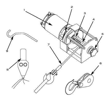
(1) Motor: 1.0 HP 12V DC motor provides power to the planetary gear mechanism.
