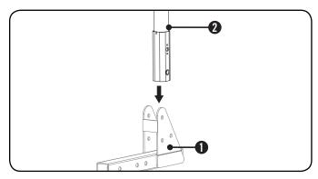
3) Secure Support Pole(2) to Square Hitch Tube(1) using a M12 x 80 Allen Bolt(15), two Ø12 Flat Washers(16) & M12 Lock Nut(18).
